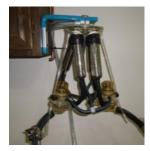
When using a Standard Cow Milker or two Goat Milkers, the CIP Unit will allow you to wash your milker unit(s) at an approximate rate of 2 gallons of wash water every 2-1/2 minutes.
