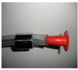
Your CIP Bucket Washer comes with 9 ft. of tubing, but you may need to shorten the length for your installation. Remove the red restrictor plug and weight, then cut tubing to desired length. Slide the weight back over the end of tubing and push the plug snugly
